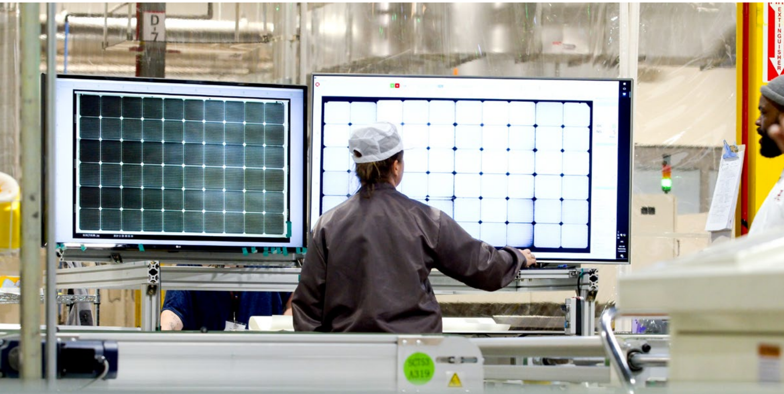
Electroluminescence (EL) image testing for micro cracks before factory shipout
